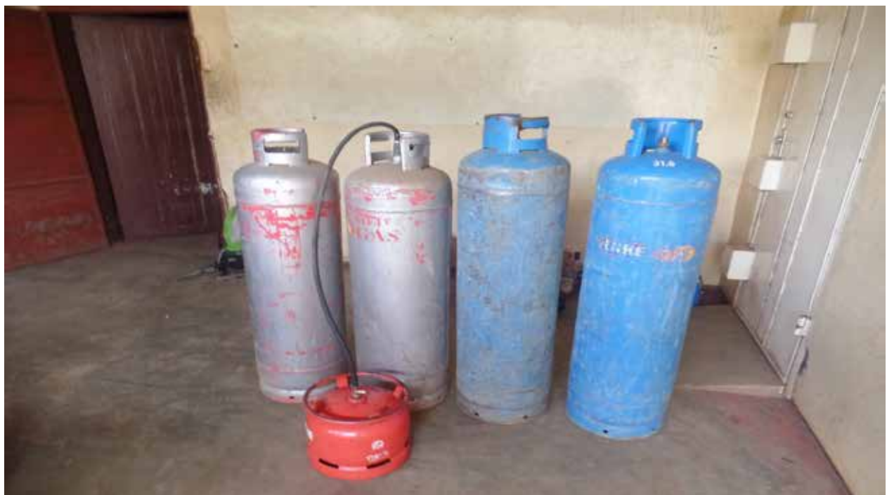
Figure 16: Flexible LPG Pipe used for illegal refilling of LPG cylinders
